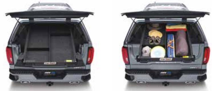
The Cap-Pack Sport is an innovative storage system that utilizes the wasted space of your truck cap to organize and secure your valuable equipment. When closed, the lightweight aluminum storage drawer locks into a sturdy elevated frame that allows your truck bed to be free of clutter and available for large items.
