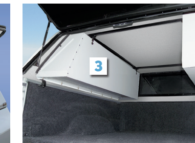
Toolboxes are securely fastened to roof framework
